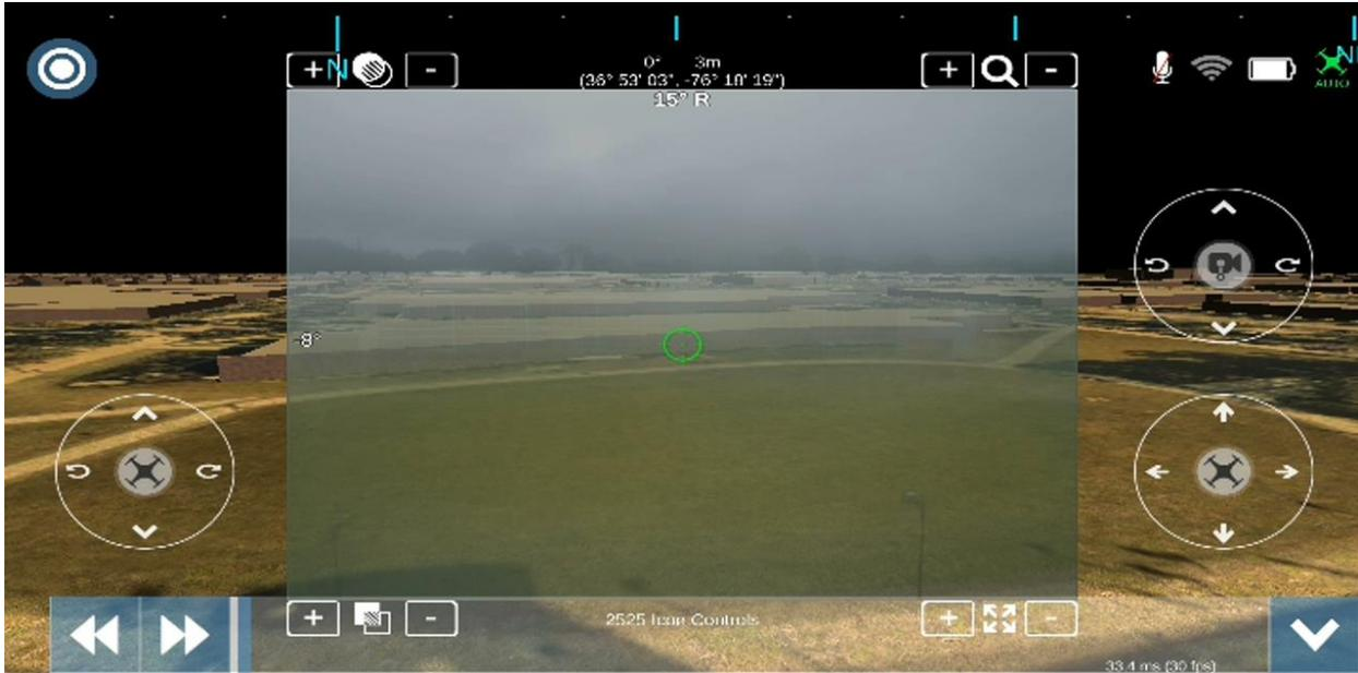
**Figure 2. FAR/SV presentation as viewed by an UAV operator with live sensor feed in the center of the FAR/SV display under degraded conditions caused by clouds and fog. Under these conditions the operator can fade the sensor image and fly using only synthetic imagery or use the surrounding synthetic imagery to support maintaining situation awareness with poor direct viewing of the environment.**
